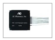
**ACP's** MS Series switch connects optical channels by redirecting an incoming optical signal into a selected output fiber. This is achieved using a patent pending opto-mechanical proprietary configuration and activated via an electrical control signal. The Switch offers ultra-high reliability and fast switching speed as well as bi-directional performance. The MS fiberoptic switches are true switching solution for optical networking applications.
